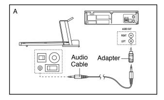
B. Plug one end of the audio cable into the jack on the front of the treadmill near the power cord. Plug the other end of the cable into the included adapter. Plug the adapter into an RCA adapter (available at electronics stores). Next, remove the wire that is currently plugged into the AUDIO OUT jack on your VCR and plug the wire into the unused side of the RCA adapter. Plug the RCA adapter into the AUDIO OUT jack on your VCR.
